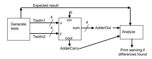
Two 4-bit inputs will be generated called *TestIn1* and *TestIn2*. These will apply every possible combination of 4-bit numbers to the *x* and *y* inputs of the adder. The value of the *sum* and *carry* outputs of the adder will be compared to our knowledge of what the outputs should be if the adder is functioning correctly. Any discrepancies will be reported during the simulation. The code for this arrangement is as follows
